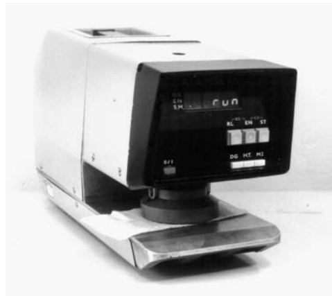
FIGURE 4.3 Example of a small mechatronic system: The ALAMBETA device for measurement of thermal properties of fabrics and plastic foils (manufactured by SENSORA, Czech Republic). It employs a unique measuring method using extra thin heat flow sensors, sample thickness measurement incorporated into a head drive, micro-processor control, and connection with a PC.
