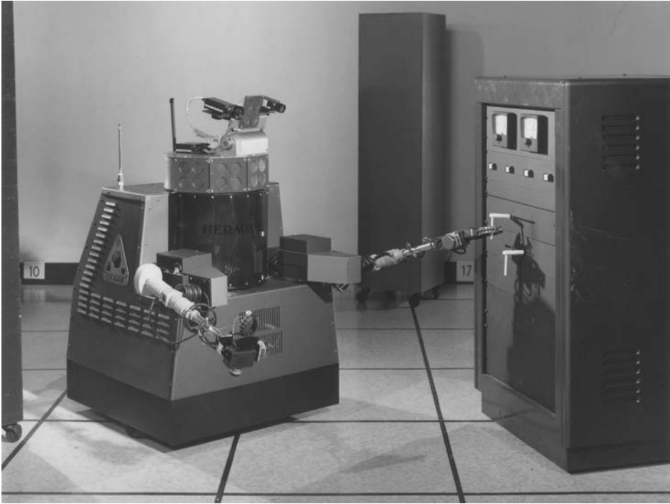
FIGURE 20.83 HERMIES IIB employed an active stereoscopic ranging system with an external laser source that could be used to designate objects of interest in the video image. (Courtesy Oak Ridge National Laboratory.)
