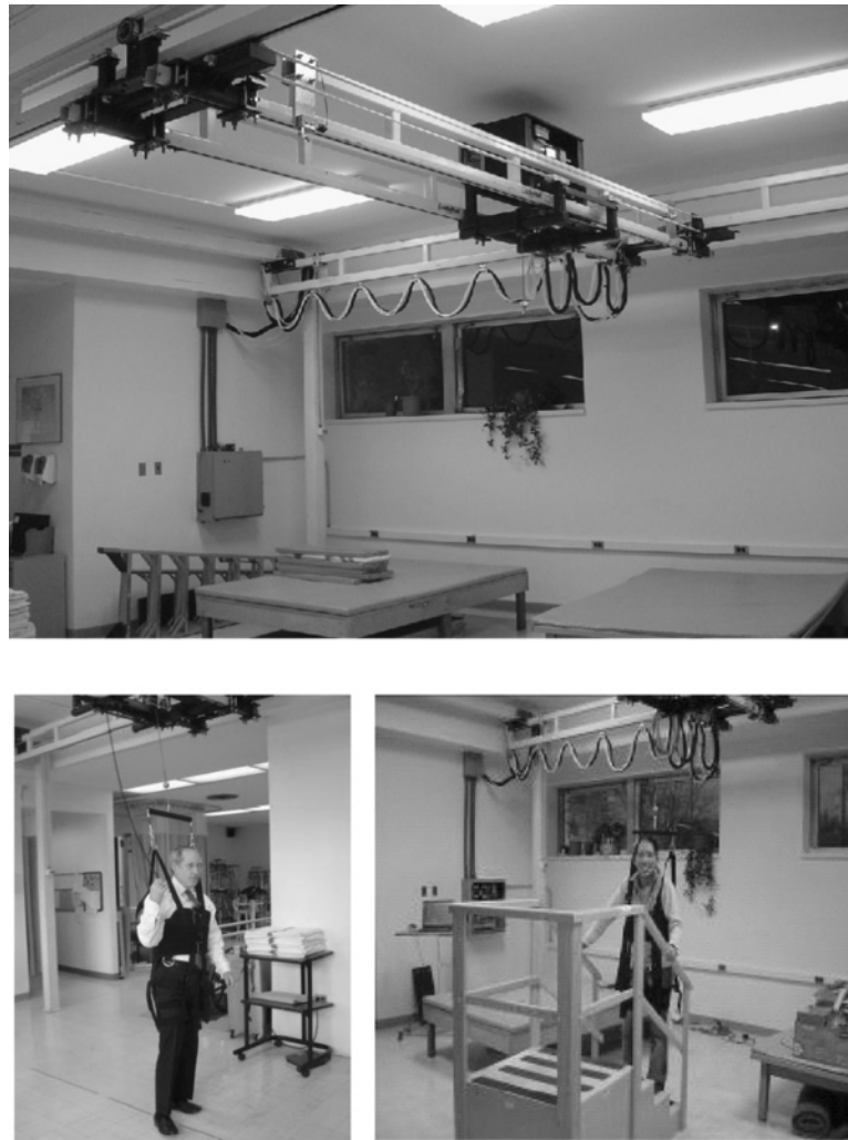
FIGURE 1-21 MECHATRONIC APPLICATION FOR REHABILITATION EQUIPMENT (COPYRIGHT US PATENT 7,462, 138B2, SHETTY, FAST AND CAMPANA)
