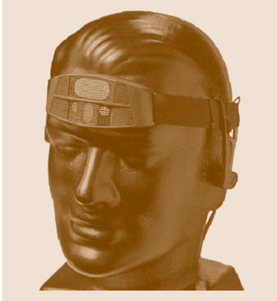
Fig. 21.22 Aid for blind people - small oval transducer is the transmitter and the other 3 are receivers. The large oval receiver provides high resolution, enabling fixation by users' fine neck control (Photo courtesy [21.54])
